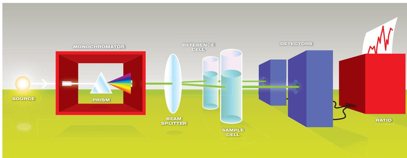
UV-visible spectrometers can be used to measure the absorbance of ultra violet or visible light by a sample, either at a single wavelength or perform a scan over a range in the spectrum. The UV region ranges from 190 to 400 nm and the visible region from 400 to 800 nm. The technique can be used both quantitatively and qualitatively. A schematic diagram of a UV-visible spectrometer is shown above.
